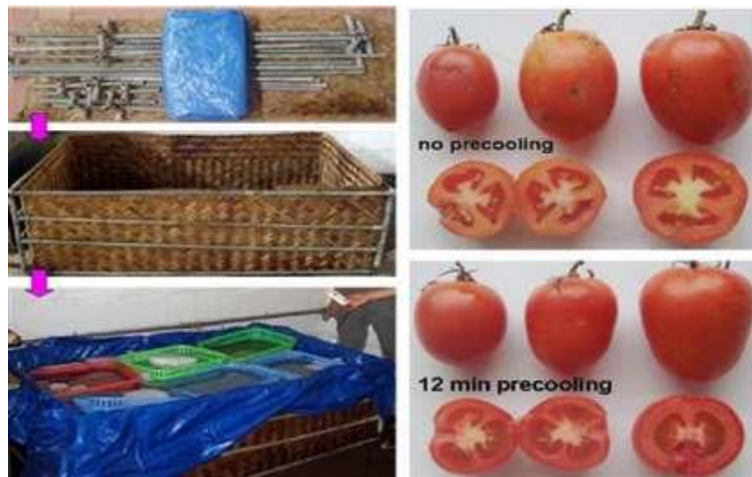
Figure 8: A simple hydro-cooler for vegetables and fruit developed at FAVRI, Vietnam, and its effect on reducing tomato chill injury (brown spots) in 10°C storage
